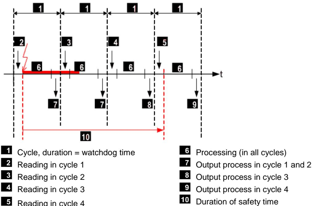
Figure 30: Transient Interference
