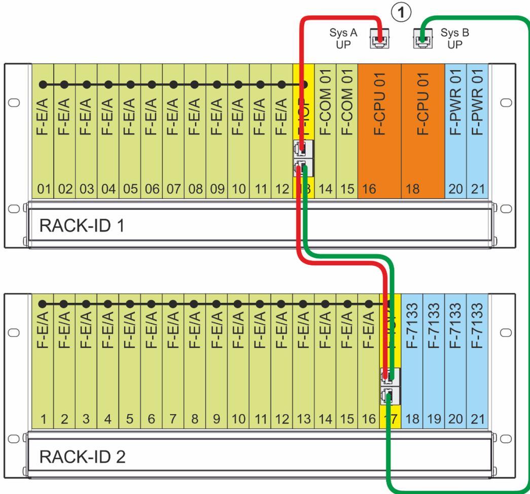
**1** System bus interfaces on the rear side of the base rack
