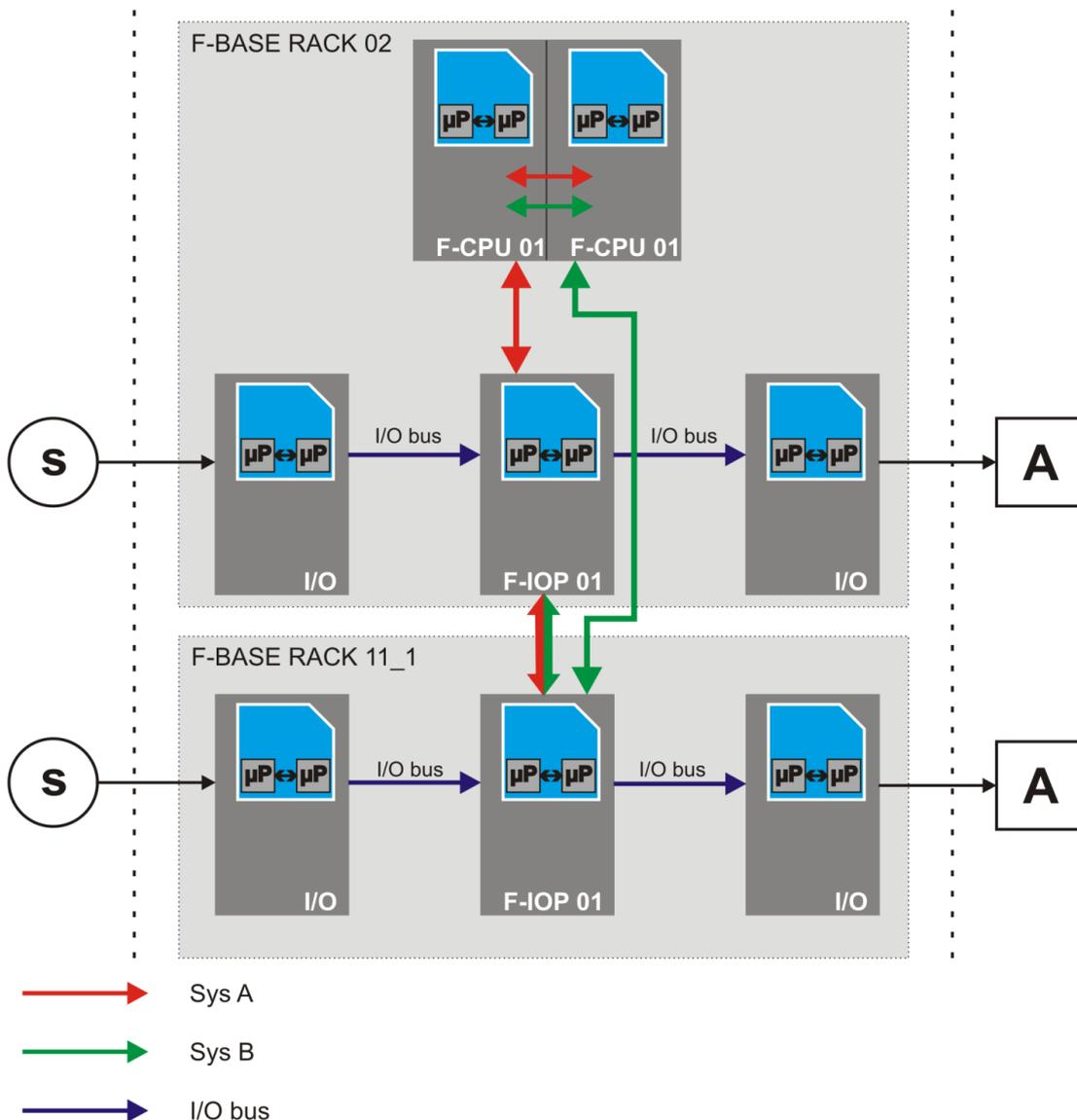
Figure 9: Example of Safe H41X Redundant Operation (1oo2)
