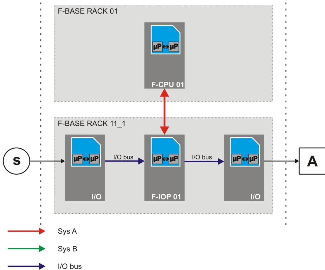
Figure 2: Example of Safe H51X Mono Operation (1oo2)
