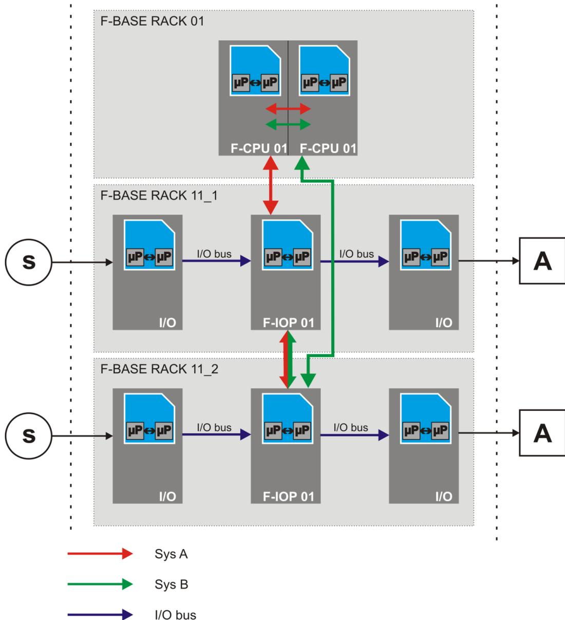
Figure 4: Example of Safe H51X Redundant Operation (1oo2)
