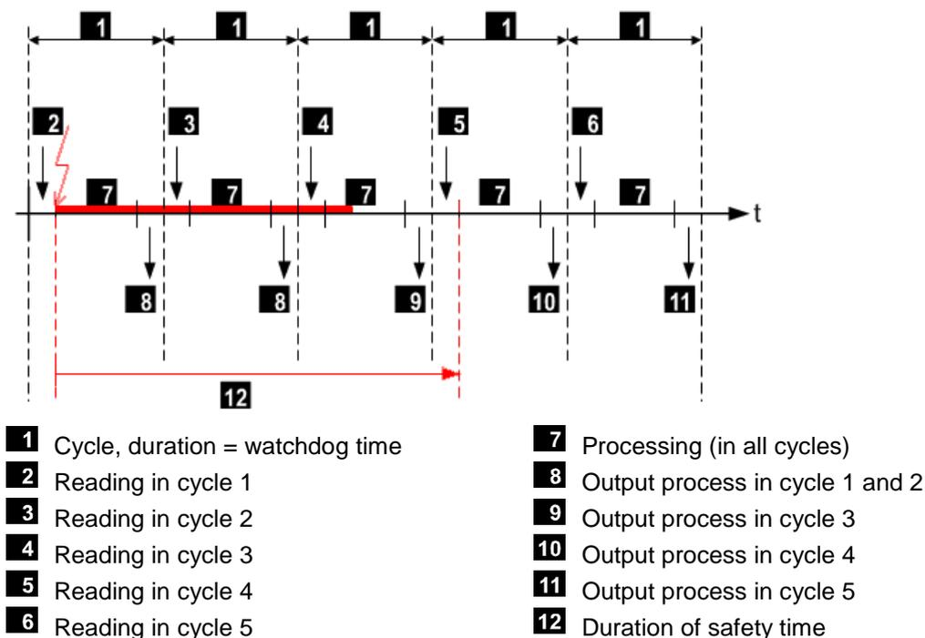
Figure 31: Interference Triggers a Safe Response
