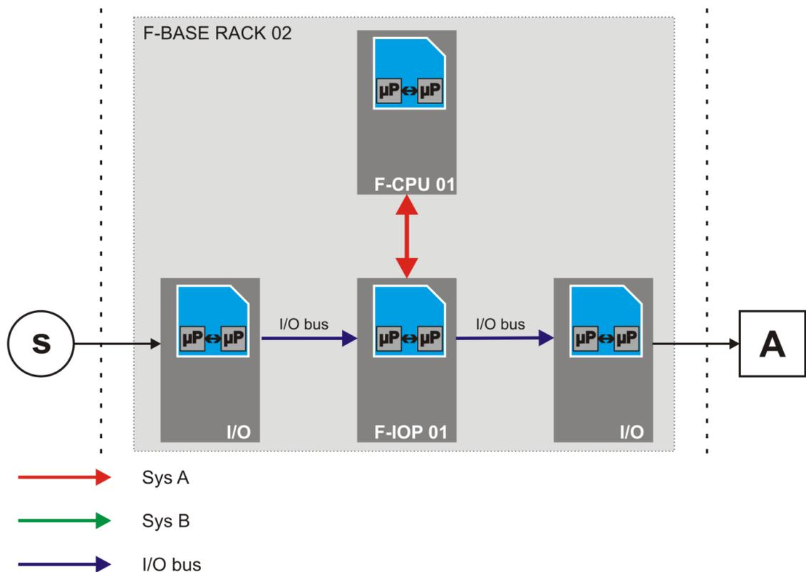
Figure 7: Example of Safe H41X Mono Operation (1oo2)
