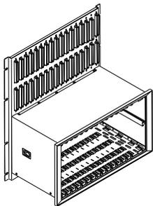
The rack depth is 349 mm (13.75 inches) and NEMA 4 and 4X weatherproof housings are available when required for environmental protection or when purge air is used.
