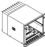
**Note:** The use of internal barriers adds 74 mm (3 inches) to the rack depth. The bulkhead-mount version of the rack is 267 mm (10.5 inches) deep. Actual dimensions of all rack types can be found in our document number 129766.
