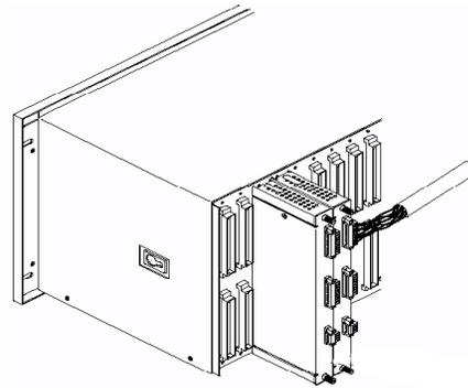
Conventional internal terminations are shown above, where field wiring terminates directly to connections on 3500 I/O modules.
